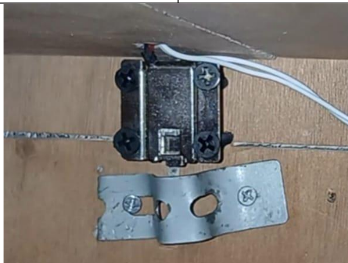
Gambar 4. 7 Solenoid Door Lock Tertarik
