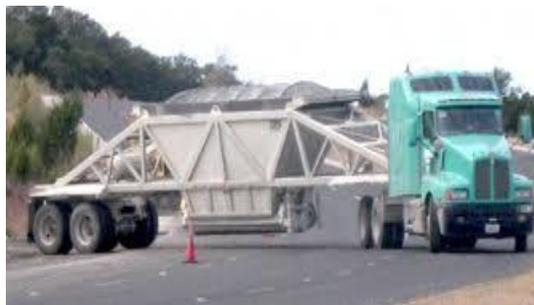
Gambar2.4 *Dump Truck Bottom Dump*
