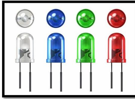
**Gambar 2.15** *Light Emitting Diode (LED)*
