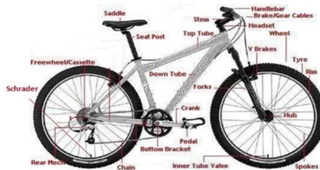
Gambar 2.2 Bagian-bagian Sepeda
