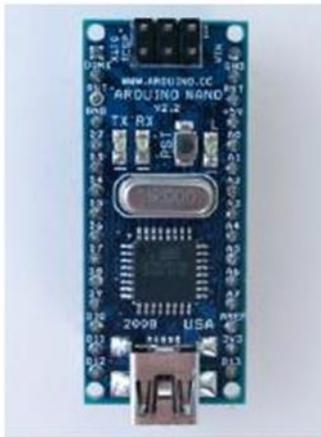
Gambar 2.7 Arduino Nano 2.x
