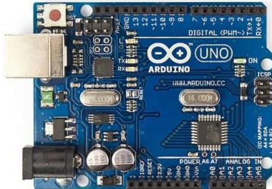
Gambar 2.8 Arduino ATmega328
