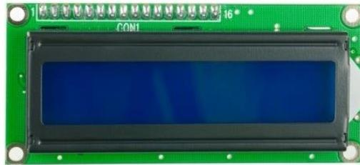
Gambar 2.18 Liquid Crystal Display 2x16
