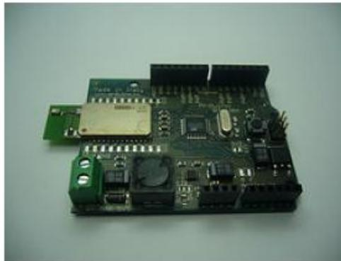
Gambar 2.6 Arduino BT (bluetooth)
