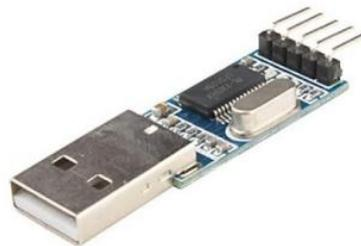
Gambar 2.9. Modul USB to TTL
