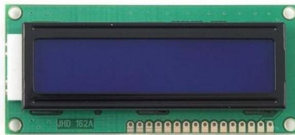
Gambar 2.14. Liquid Crystal Display 2x16
