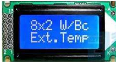
Gambar 2.3 LCD 8x2
