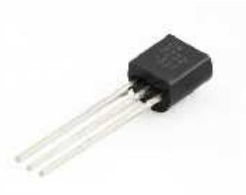
Gambar 2.8. Transistor
