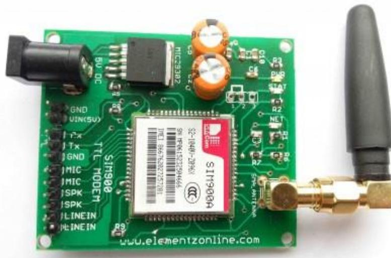
**Gambar 2.5 Modem GSM SIM900A**
