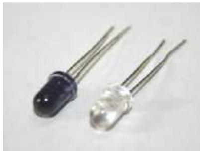
**Gambar 2.2 LED infrared**
