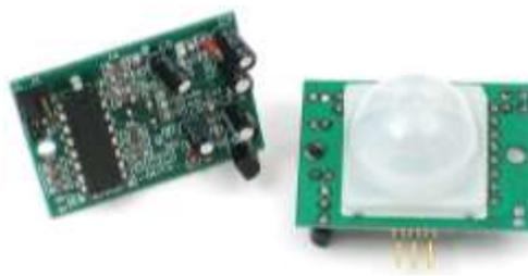
**Gambar 2.3 Module Sensor PIR HCSR501**
