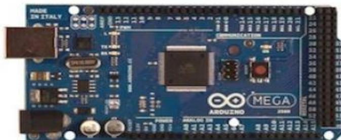
Gambar 2.4 Arduino Mega 2560
