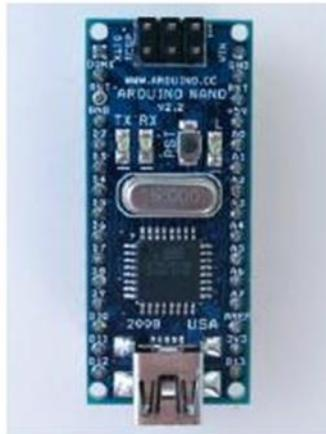
Gambar 2.8 Arduino Nano 2.x
