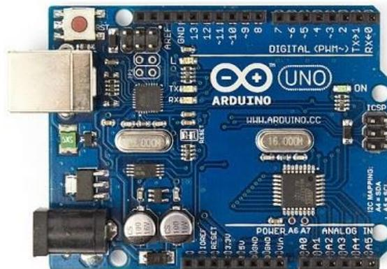
Gambar 2.9 Arduino ATmega328
