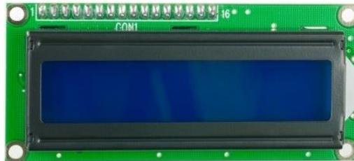
Gambar 2.19 Liquid Crystal Display 2x16
