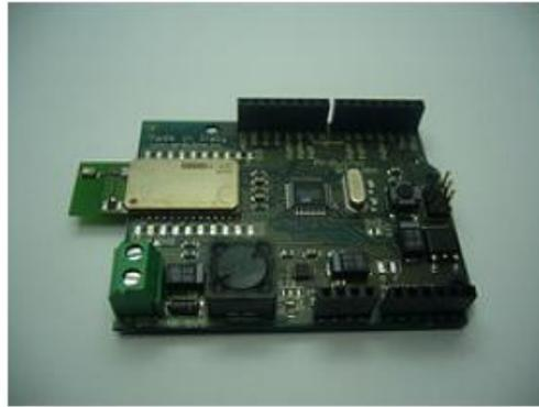
Gambar 2.7 Arduino BT (bluetooth)
