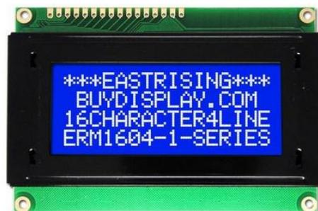
**Gambar 2.9** Liquid Crystal Display 16x4
