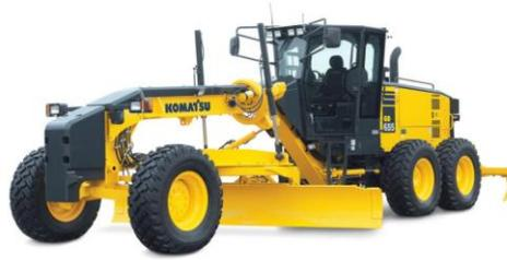
Gambar. 2.3 Motor grader
