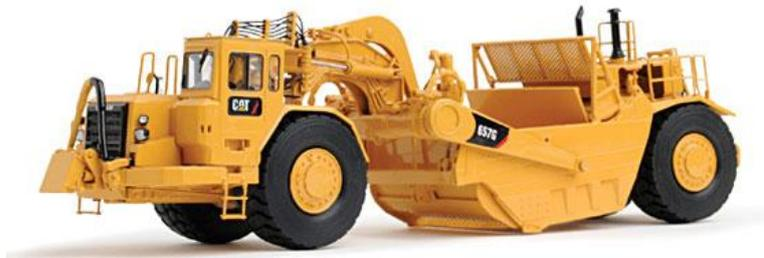
Gambar. 2.4 Wheel Tractor Scraper
