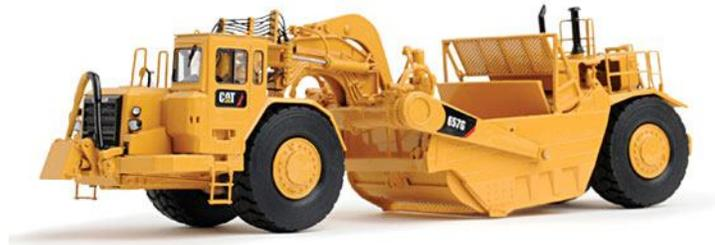
**Gambar. 2.4** *Wheel Tractor Scrapper*
