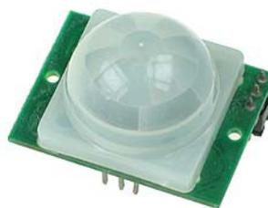
**Gambar 2.9 Sensor Gerak PIR**
