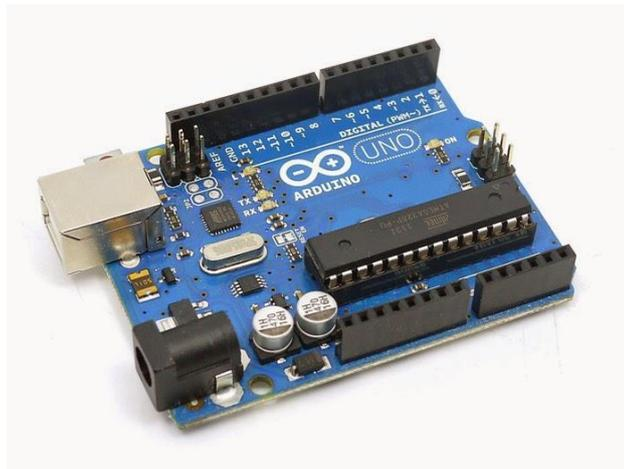
**Gambar 2.5** Modul Arduino Uno
