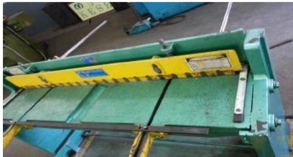
Gambar 2.20 Mesin Potong Guillotine Pedal
