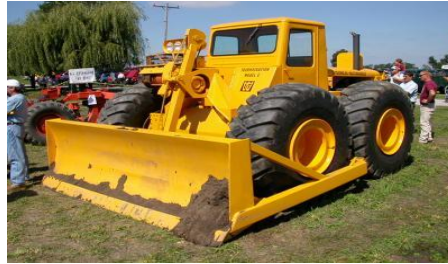
Gambar 2.3 Wheel Tractor Dozer
