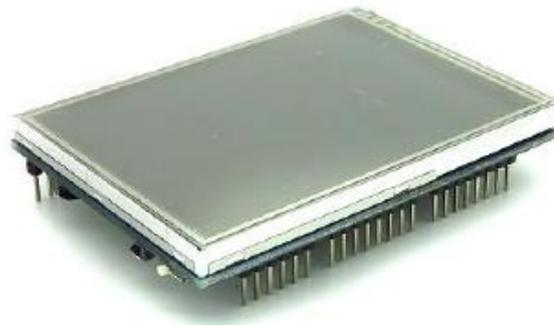
**Gambar 2.9** LCD TFT
