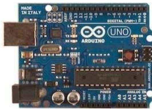
Gambar 2.24 Board *Arduino Uno*
