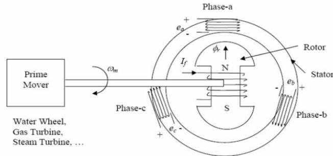
Gambar 2.2 Prinsip Kerja Generator Sinkron<sup>2</sup>
