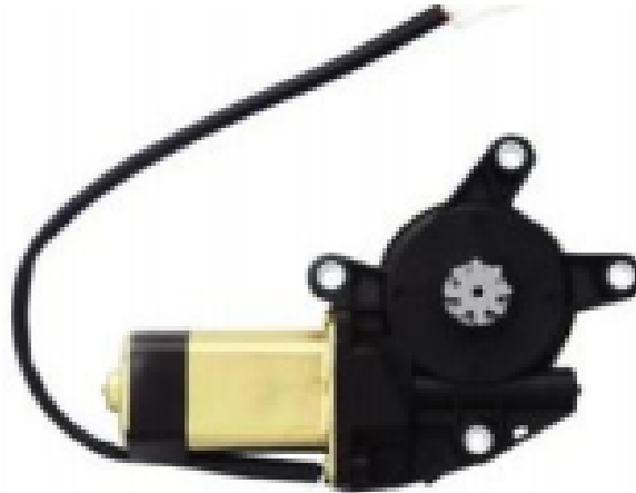
Gambar 2.7 Motor DC Power Window
