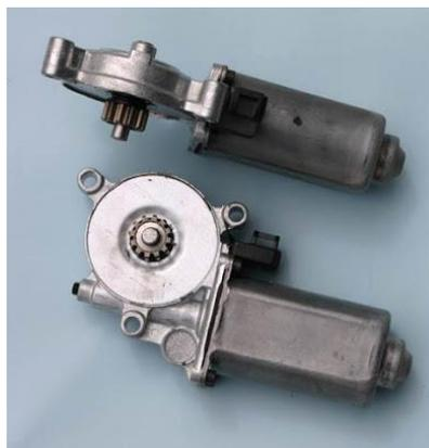
**Gambar 2.5 Motor DC 12 Volt DC / 30Kg**
