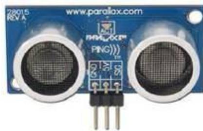
**Gambar 2.3** Sensor Ping ultrasonik
