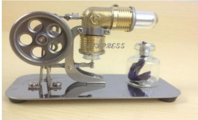
Gambar 5. *Stirling Engine* Tipe Beta
