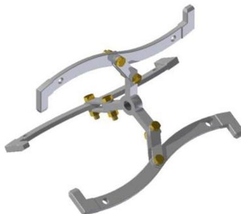
Gambar 2.7: *Puller bearing*
