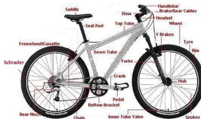
Gambar 2.2 Bagian-bagian Sepeda
