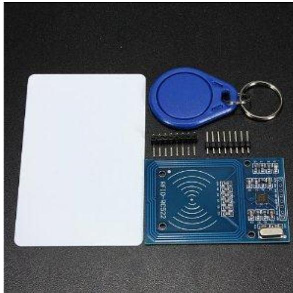
**Gambar 2.8** Modul RFID RC-522
