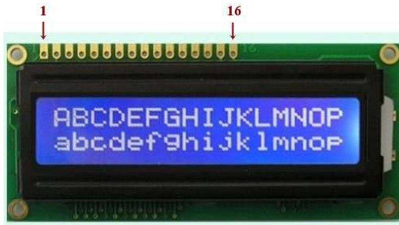
**Gambar 2.12** Liquid Crystal Display (LCD)
