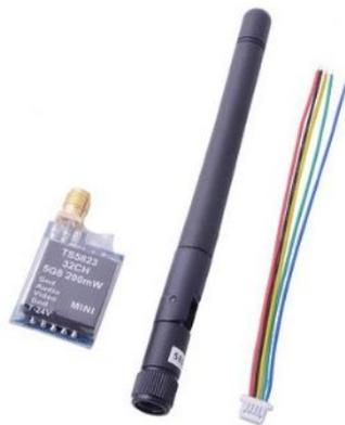
Gambar 2.12 Transmitter TS5823
