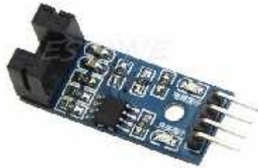
**Gambar 2.23** Modul Sensor *Optocoupler*
