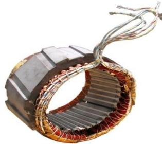
Gambar 2.4 Stator (sumber: <http://pravivefenee.blog.com/2011/11/30/stator-coil-rewinding>)
