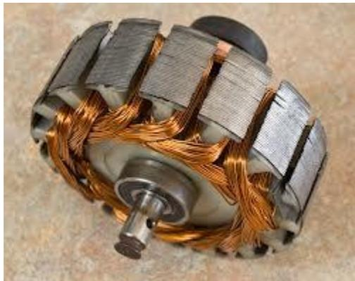
Gambar 2.3 Rotor (sumber: <http://www.electricaleasy.com/2012/12/basic-construction-and-working-of-dc.html>)
