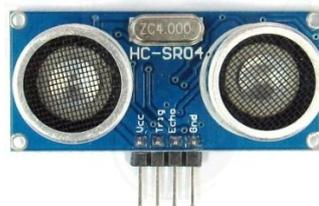
**Gambar 2.4** Sensor Ultrasonik HC-SR04
