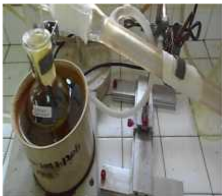
Gambar 5. Proses Distilasi Lipid Mikroalga
