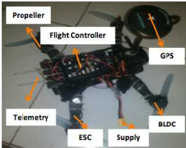
Fig. 4. The position of components in UAV
