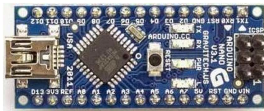
**Gambar 2.10** Arduino Nano R3
