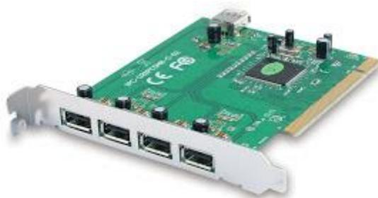
**Gambar 2.22** Internal USB PCI Card
