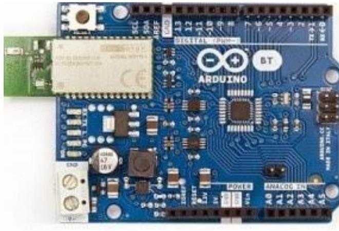
**Gambar 2.18** Arduino BT
