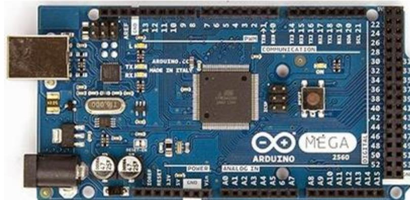
**Gambar 2.7** Arduino Mega2560
