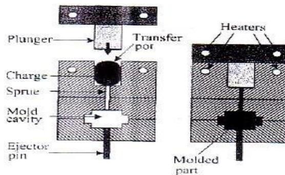
**Gambar 2.4 Proses compression moulding**
