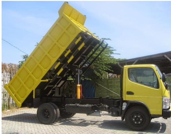
Gambar 2.2 *Dump Truck with Rear Dump*
