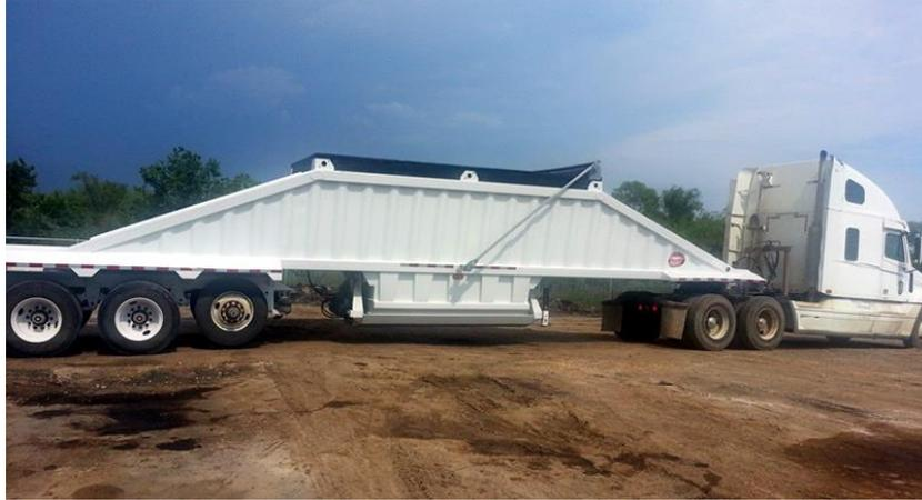
Gambar2.4 *Dump Truck with Bottom Dump*
