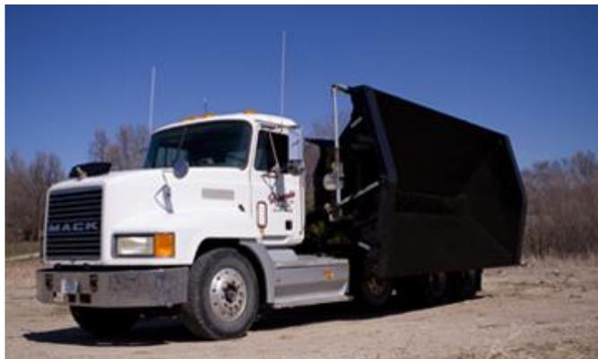
Gambar 2.3 *Dump Truck with Side Dump*
