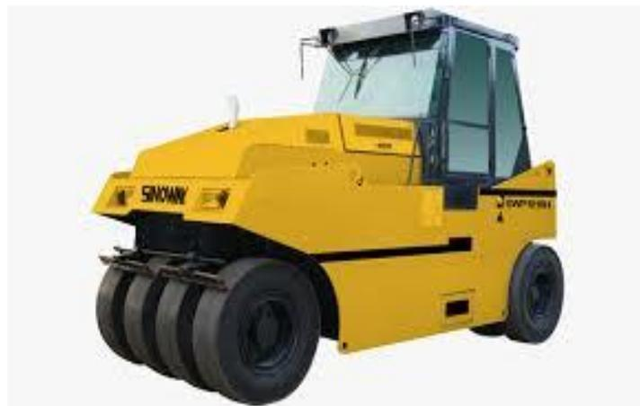
Gambar 2.6 *Pneumatic Tired Roller*
