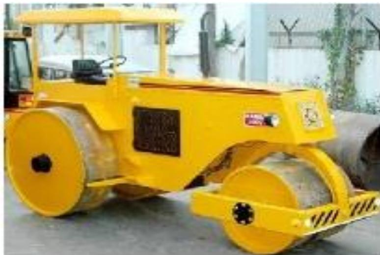
Gambar 2.2 *Three Wheel Rollers*
