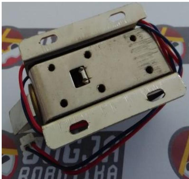
Gambar 2.6. Gambar *electric door lock*
