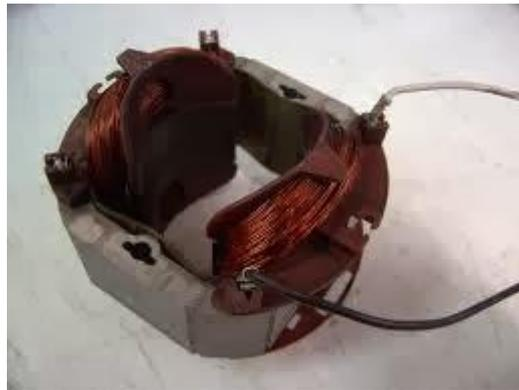
Gambar 2.6 stator motor universal
