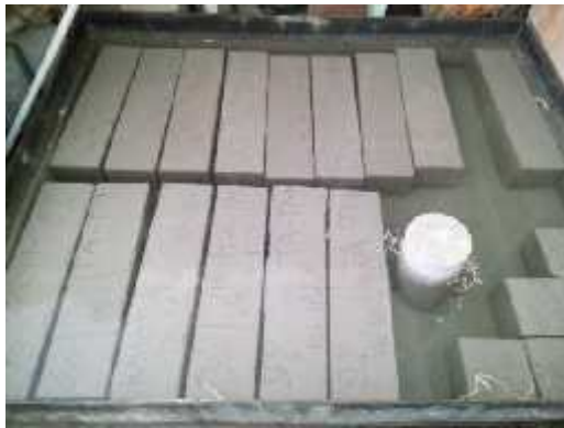
Gambar 18 : Proses perendaman sampel beton
