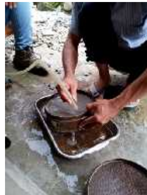
Gambar 11: Pengujian Kadar Lumpur
