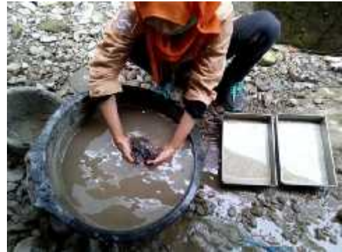
Gambar 6 : Pencucian Agregat Kasar
