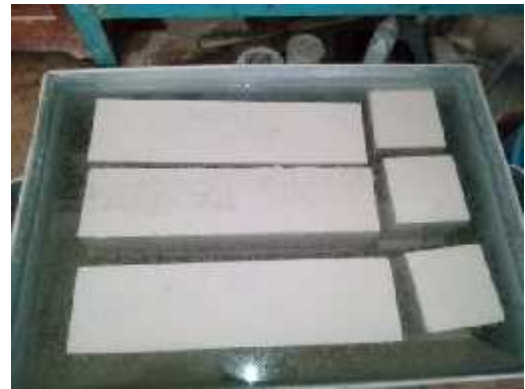
Gambar 18 : Proses perendaman sampel beton
