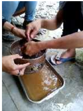
Gambar 11: Pengujian Kadar Lumpur
