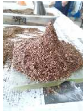
Gambar 10: Pengujian SSD ( Saturated Surface Dry ) Agregat Halus
