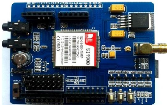
*Gambar 2.4 GSM Shield Icomsat V1.1 SIM 900*
