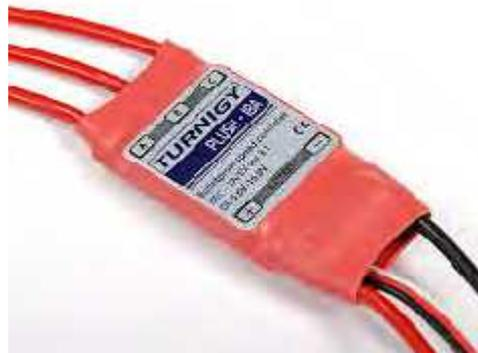
**Gambar 2.10** Electronic Speed Controller
