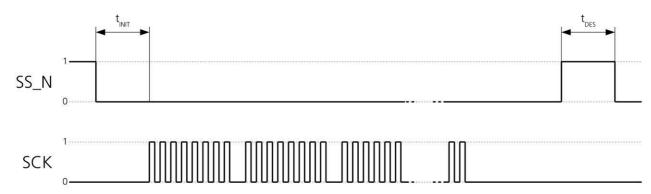
Figure 3: SPI timing diagram
