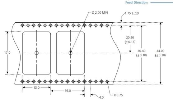
Figure 5: Dimensions and orientation for NEO-M8 modules on tape
