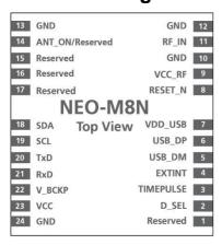
Figure 2: Pin Assignment
