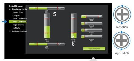
Select Radio Calibration to teach Pixhawk to work with your RC transmitter. Turn on your transmitter, select Calibrate Radio, and move all sticks and switches to their extreme positions. Select Click when Done once the red bars are set for all available channels.
