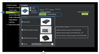
Select the options to enable the compass; to allow automatic declination calculation; and to specify Pixhawk. Select Live Calibration to launch the wizard, and follow the prompts.
