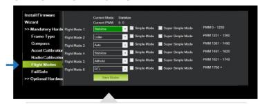
Move each switch on your transmitter to its available positions. The mission planner will indicate the currently selected position with green highlighting. Select a mode for each switch position, and select Save Modes to assign.
