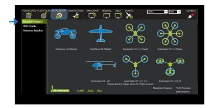
When prompted, follow the directions to load the firmware. Once the status bar shows that the download is complete, power cycle the board by disconnecting and reconnecting the USB.
