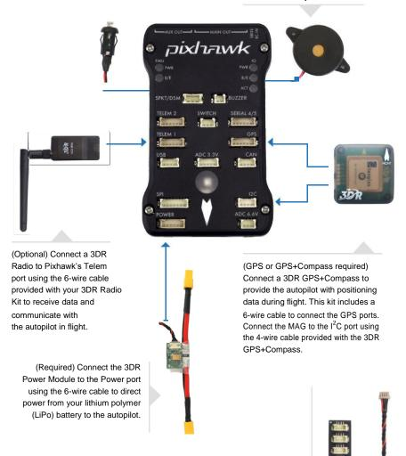
(Optional) The I<sup>2</sup>C splitter expands the I<sup>2</sup>C port to allow up to four additional peripherals to connect to Pixhawk. Use the 4-wire cable to connect the I<sup>2</sup>C splitter and add a compass module, external LED, digital airspeed sensor, or other peripherals to your vehicle.
