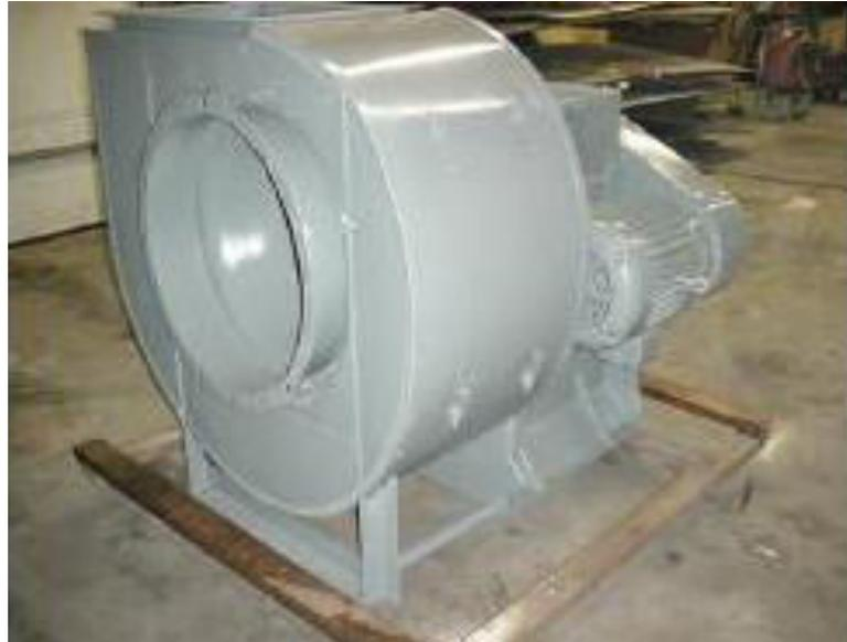
Gambar 2.10 Blower Sentrifugal (*Fan Air Company*)
