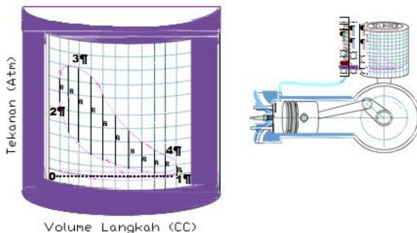
**Gambar 2.13 Diagram Indikator Motor**
