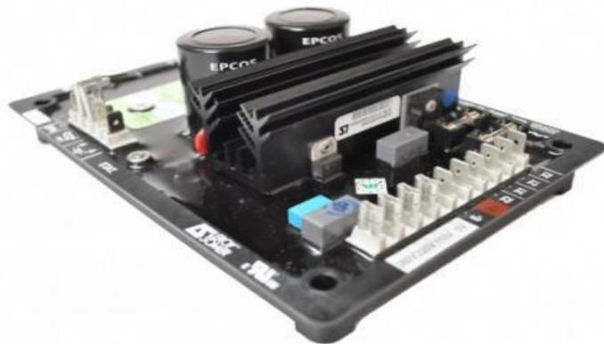
**Gambar 2.18 Automatic Voltage Regulator ( AVR )**
