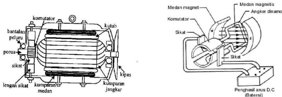
**Gambar 2.3 Motor Listrik DC (*Electrical Engineering: Principles and Applications, 5e*, by Allan R. Hambley)**
