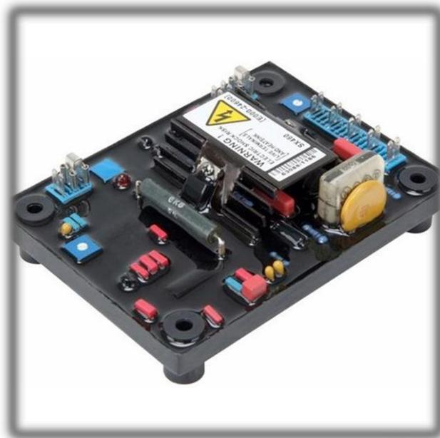
**Gambar 2.22 Automatic Regulator Voltage**
