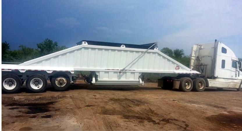
Gambar2.4 *Dump Truck with Bottom Dump*
