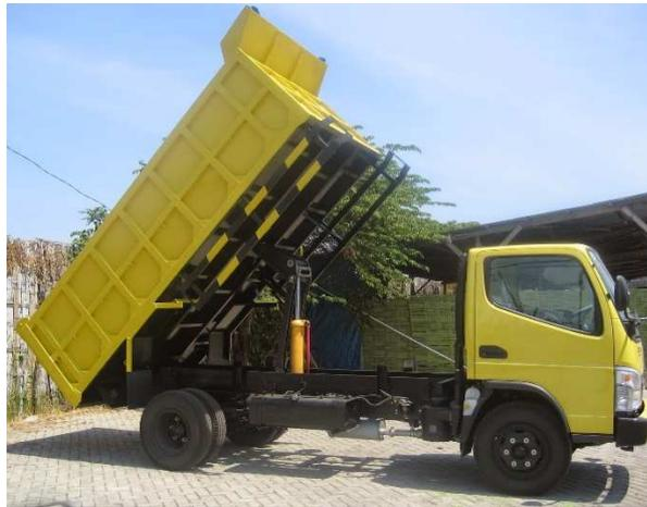
Gambar 2.2 *Dump Truck with Rear Dump*
