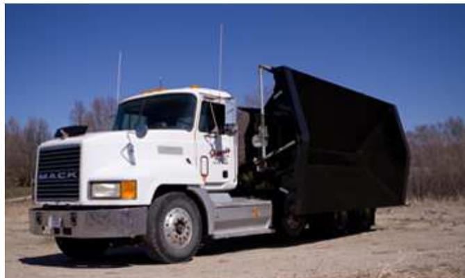
Gambar 2.3 *Dump Truck with Side Dump*
