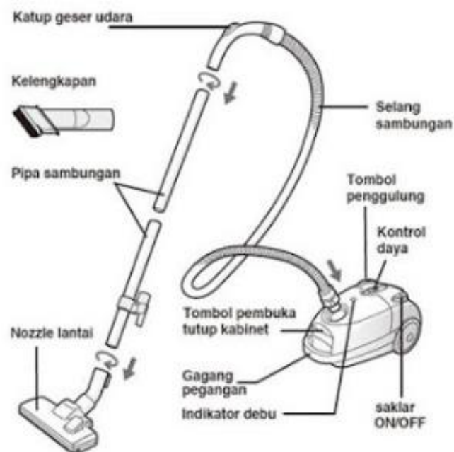
Gambar 2.1 bagian – bagian vacuum cleaner
